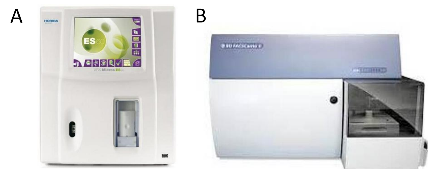
Figure 2: Instruments used to perform the immune cell profile. A) The Hematology analyzer ABX Micros ES 60 (Horiba) was used to know the number of monocytes and granulocytes of healthy donors; B) The flow cytometer BD FACSCanto II (BD) was used to perform the T cell phenotyping for both healthy donors and PsA patients
